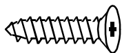
#12 X 1" (min.) SHEET METAL SCREW INTO JAMB (FURNISHED BY TIGER DOOR FOR BUTT HINGES, FURNISHED BY HINGE MANUFACTURER FOR CONTINUOUS HINGE)
