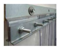
are constructed of 14 gauge galvanized steel with 1/4" studs. Face plates are formed in 12" sections for easy strip replacement. The steel face plate holds strips firmly while allowing flex without breaking.
