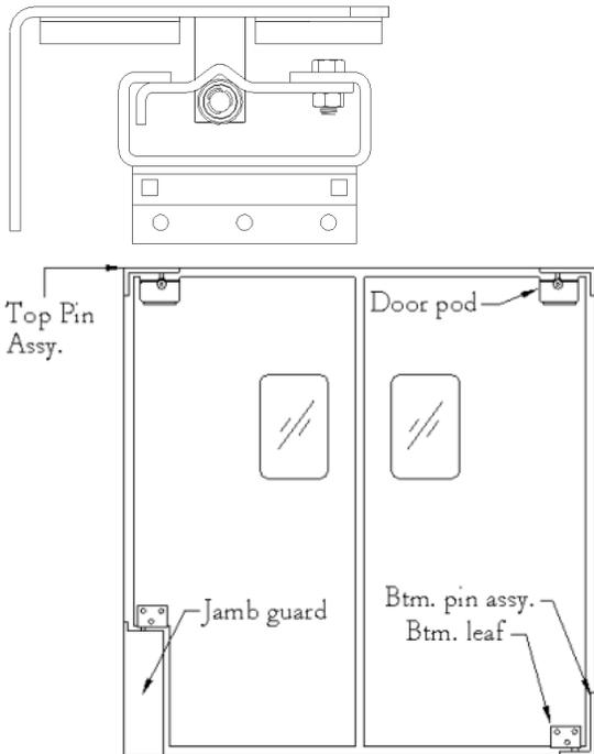
NOTE: Bottom pin assembly must be secured to floor.
